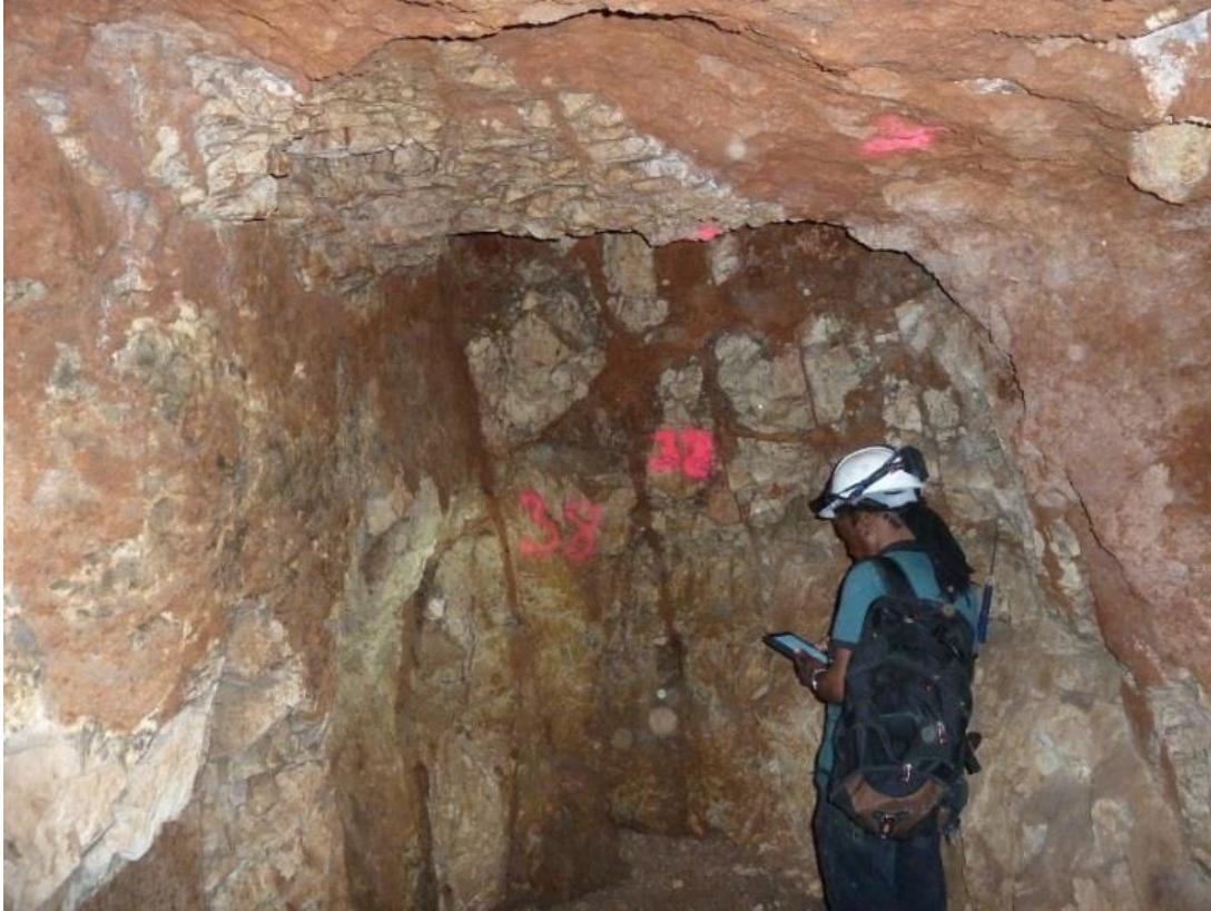
Figure 7: Photograph of a cross-cut on the 50' level in the Christiana Mine ending in descloizite-bearing breccia mineralisation. Note the stable ground conditions of the historical workings.
