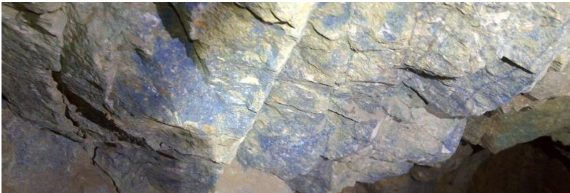
Figure 5: Azurite mineralisation in underground exposure at Nosib Block Mine
