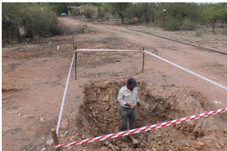
Figure 2: Pit dug to 1m into surface mineralised material comprising old stockpile material and tails near the Abenab open pit
