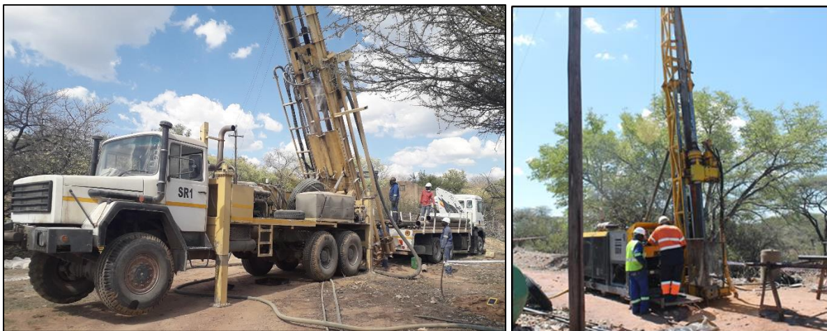
Figure 5-6: RC and diamond drill rigs in operation at the Abenab Mine.
