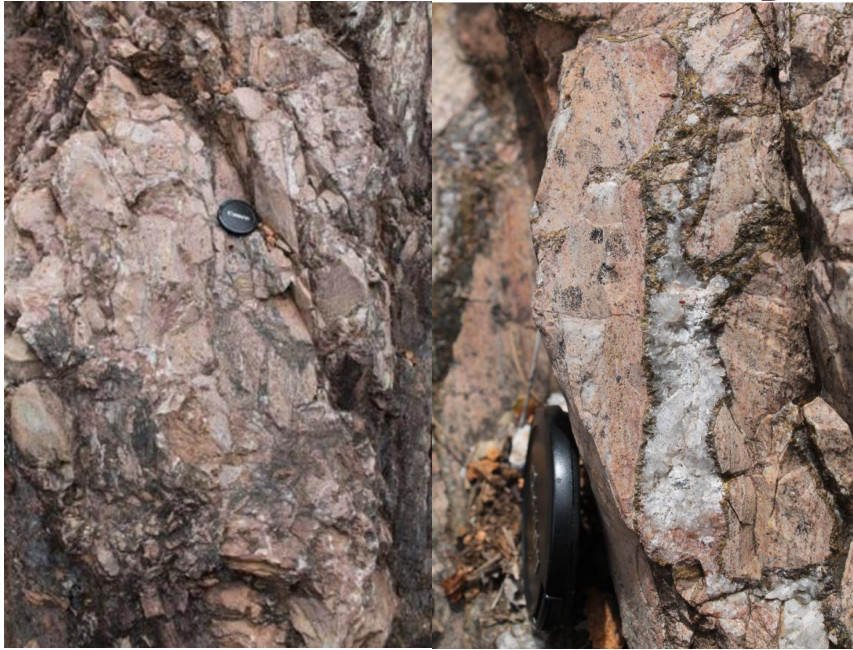
Figure 2: Brecciated limestone with calcite-descloizite fracture fill in the south wall of the Abenab pit
