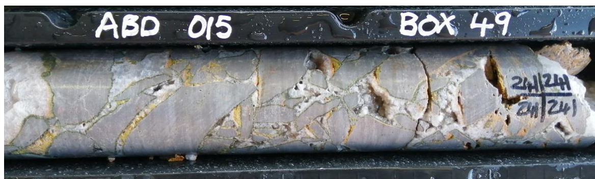
Figure 8: Dolomite breccia with grey-green descloizite (vanadium) mineralisation lining calcite filled fractures in diamond hole ABD015 at 241m
