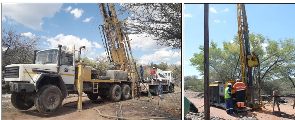
Figure 3-4: RC and diamond drill rigs in operation at the Abenab Mine.
