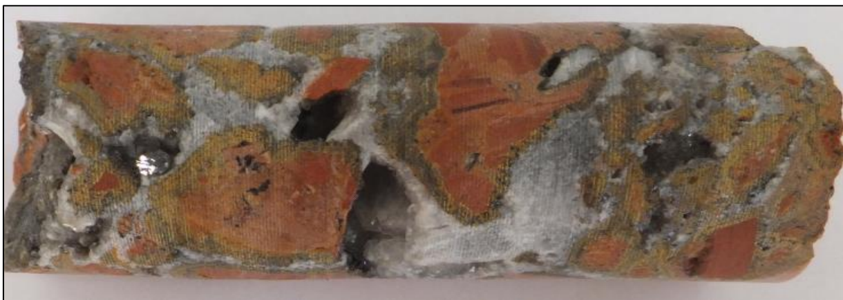
Figure 5: Vanadium bearing breccia in diamond hole 241.98m in ABD014. Dolomite clasts - red brown, descloisite – yellow brown, spar calcite – white
