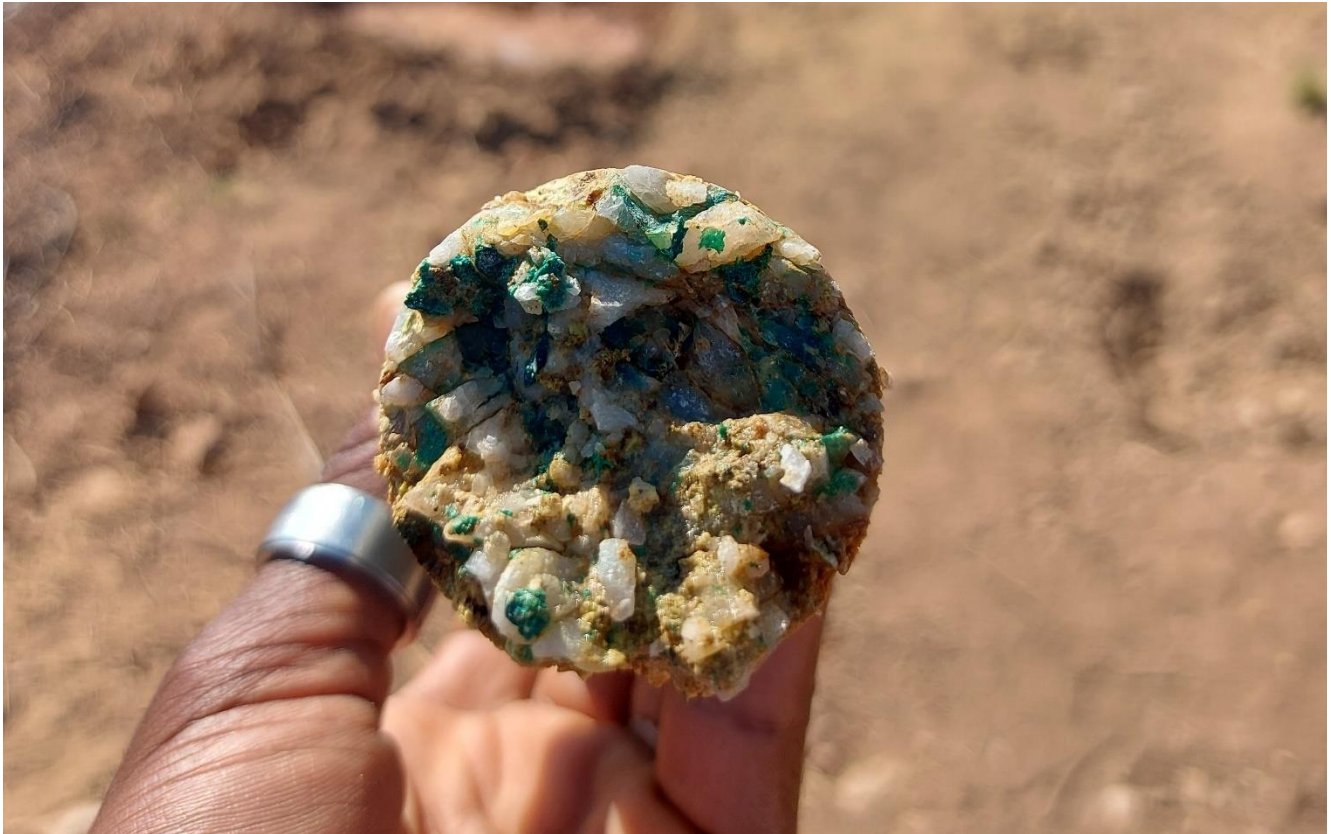
Photo 1: Diamond drill-core from Nosib Block Prospect, NSBDD001, malachite at approximately 12m down-hole
