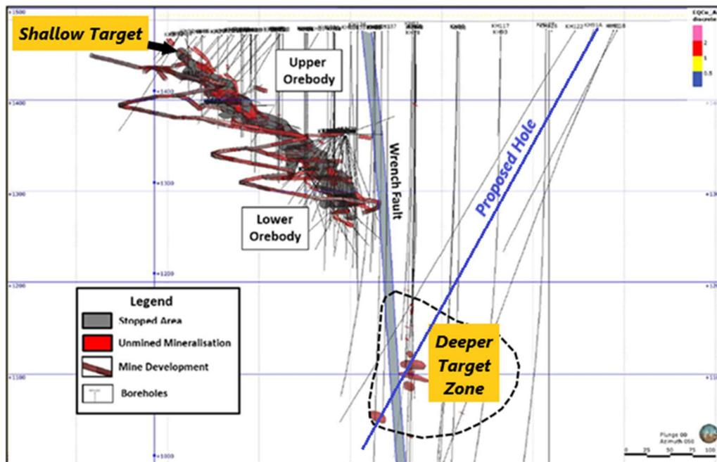
**Figure 5:** Cross section of Khusib Springs Mine showing developed and stope areas, un-mined zones, and targets.
