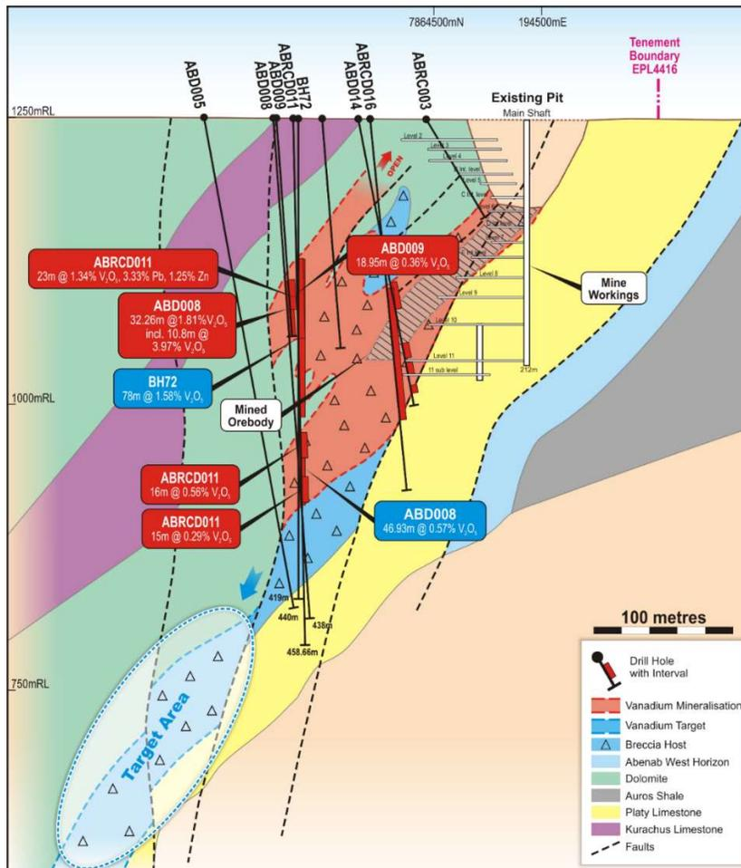
**Figure 2: Cross section through Abenab breccia showing previous workings, 2019 drilling and high-grade vanadium mineralisation (looking east).**
