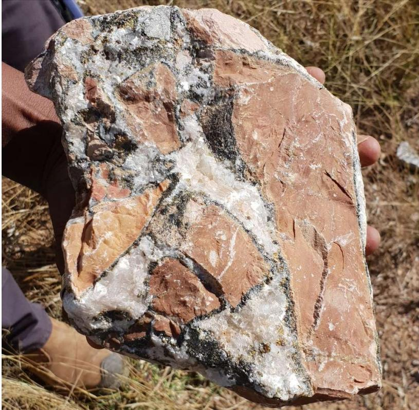
**Photo 1: Abenab Breccia with descloisite crystals (black) rimming brecciated dolomite fragments.**
