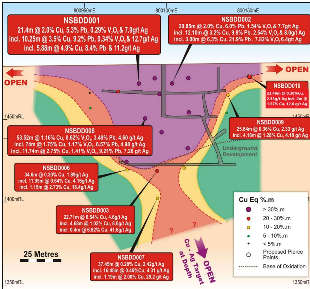
**Figure 4: Nosib Prospect, longitudinal projection with NSBDD008 and other key intersections.**
