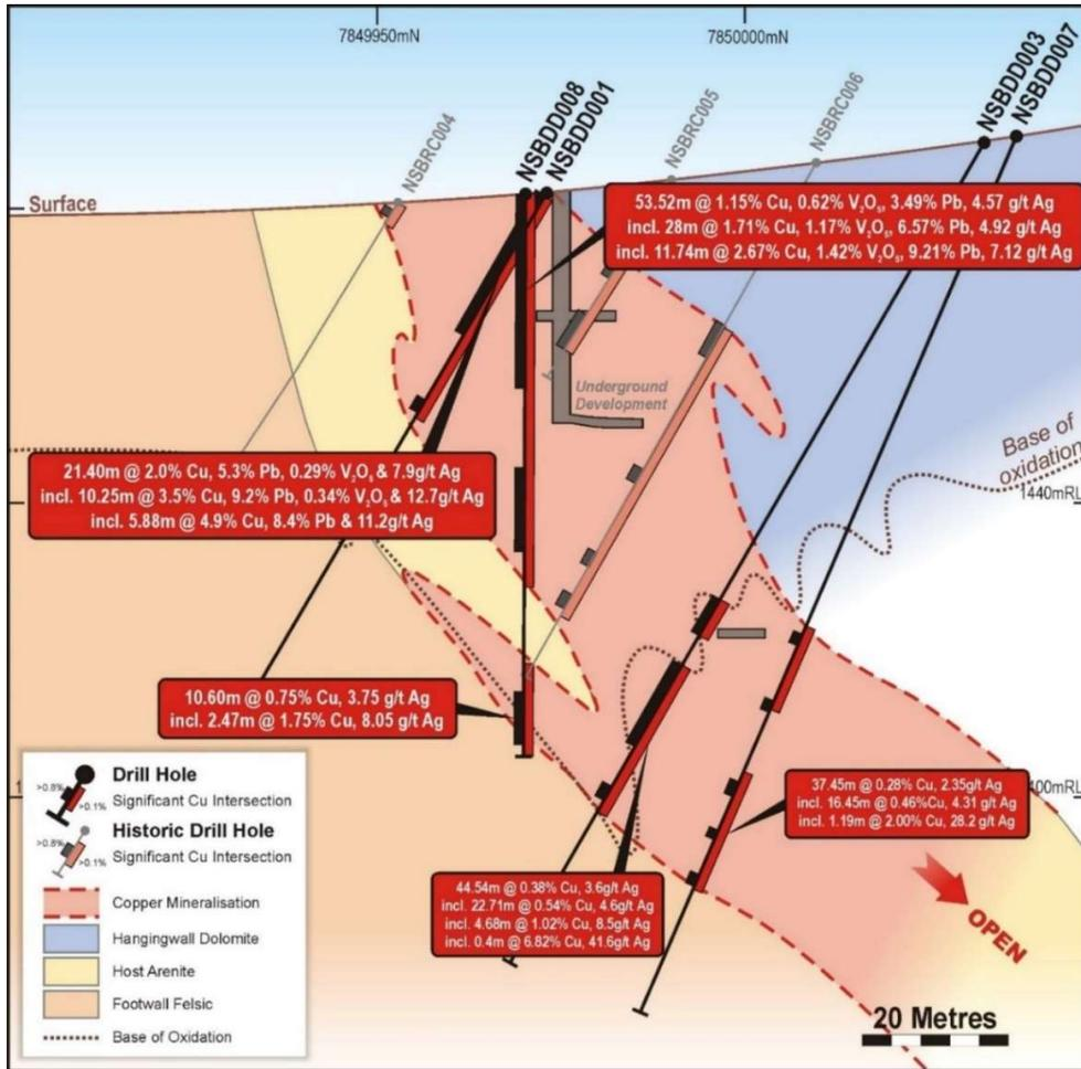
Samples of diamond drill-core from NSBDD008 at Nosib with other previous intersections (e.g., NSBDD002<sup>2</sup>) and material from a recent bulk sample excavated from the top of the Nosib supergene mineralisation (see Photo 2 below) have been aggregated to produce a bulk sample for gravity concentration testwork based on the flow-sheet developed for the Abenab resource material. This will aim to generate >5kg of concentrate, targeting a 10 to 15 times upgrade of vanadium, lead and copper.
