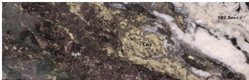
HVD003, 102.3 - 102.5m semi-massive chalcopyrite and sphalerite
